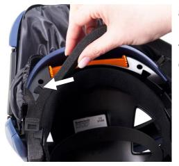
**8.3** Fit the new forehead seal. Press down the tabs of the forehead seal in the socket on the face shield.
