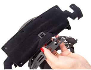
**9.2** Push in the head harness tongue into the new sweatband. Note how the sweatband is turned!
