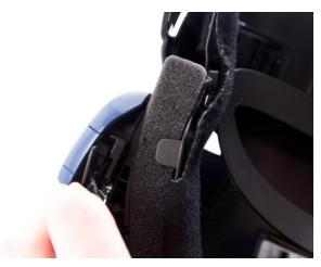
**7.2** Push the face seal pins out and remove the face seal.
