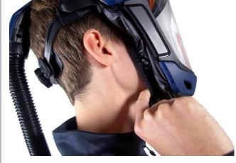
4.3 Insert a finger between your chin and the face seal and run the finger along the contact surface of the face seal all the way round to check that it fits well against the face.
